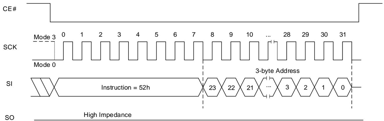
**Figure 8.19 Block Erase (32K) QPI Sequence**
