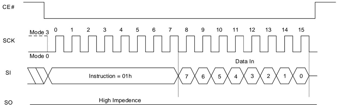
**Figure 8.29 Write Status Register QPI Sequence**
