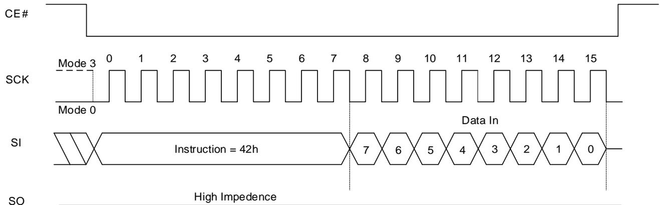
**Figure 8.33 Write Function Register QPI Sequence**
