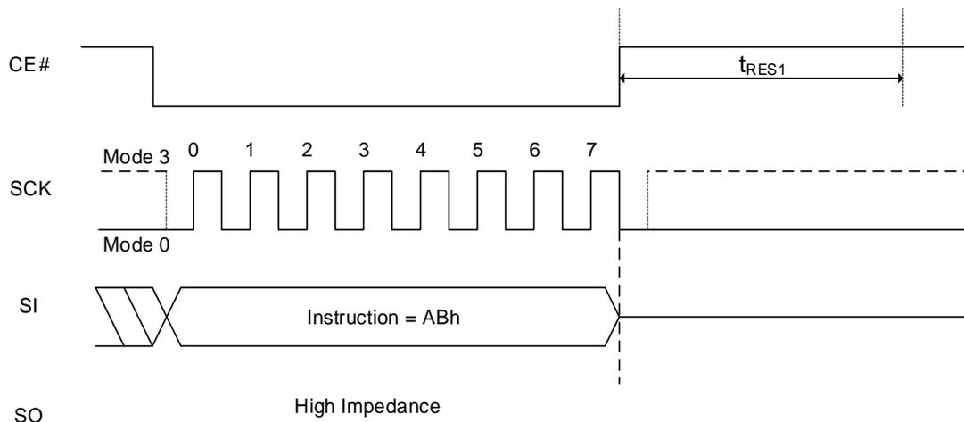
**Figure 8.39 Release Power Down QPI Sequence**
