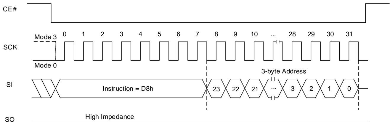
**Figure 8.17 Block Erase (64K) QPI Sequence**
