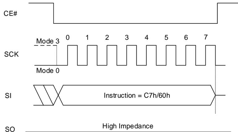
**Figure 8.21 Chip Erase QPI Sequence**
