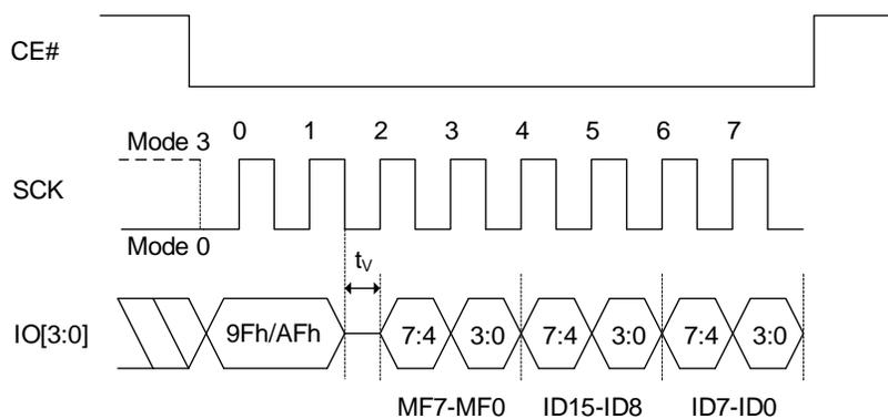
**8.27 READ DEVICE MANUFACTURER AND DEVICE ID OPERATION (RDMDID, 90h)**
