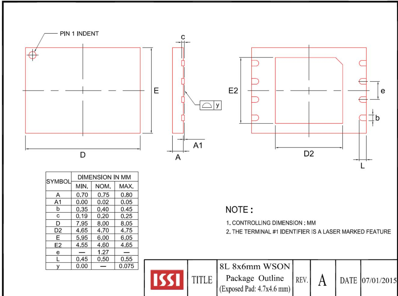
Note: All dimensions are in millimeters. Lead co-planarity is 0.08mm.
