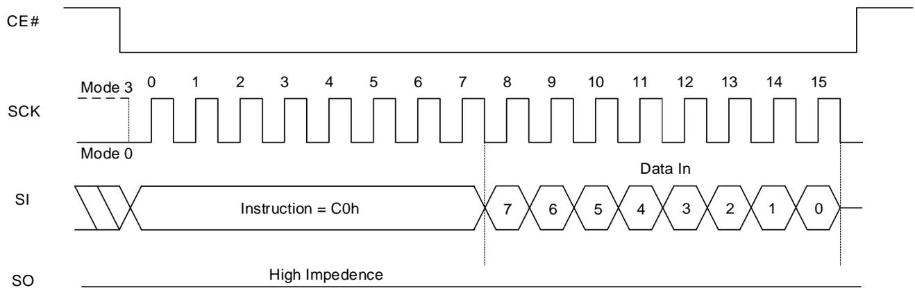
**Figure 8.41 Set Read Parameters QPI Sequence**
