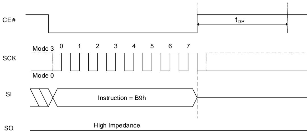
**Figure 8.37 Enter Deep Power Down Mode QPI Sequence**
