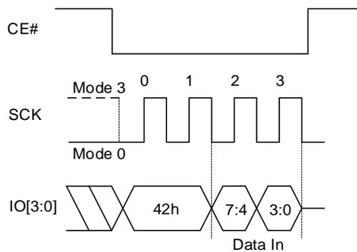
**8.20 ENTER QUAD PERIPHERAL INTERFACE (QPI) MODE OPERATION (QPIEN, 35h; QPIDI, F5h)**
