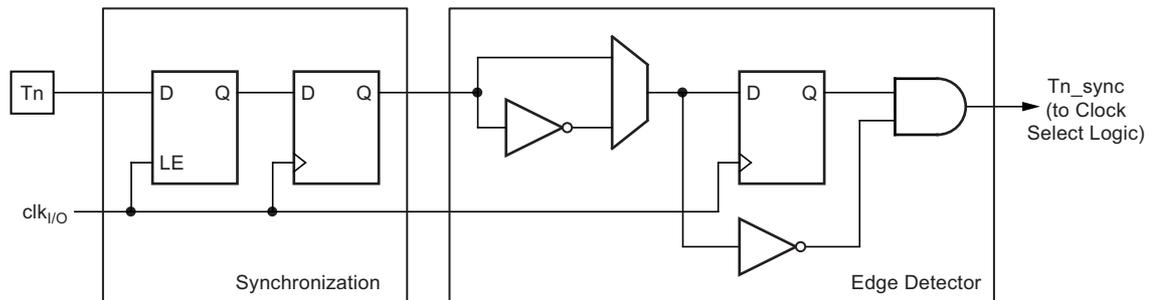
The synchronization and edge detector logic introduces a delay of 2.5 to 3.5 system clock cycles from an edge has been applied to the  $Tn/T0$  pin to the counter is updated.
