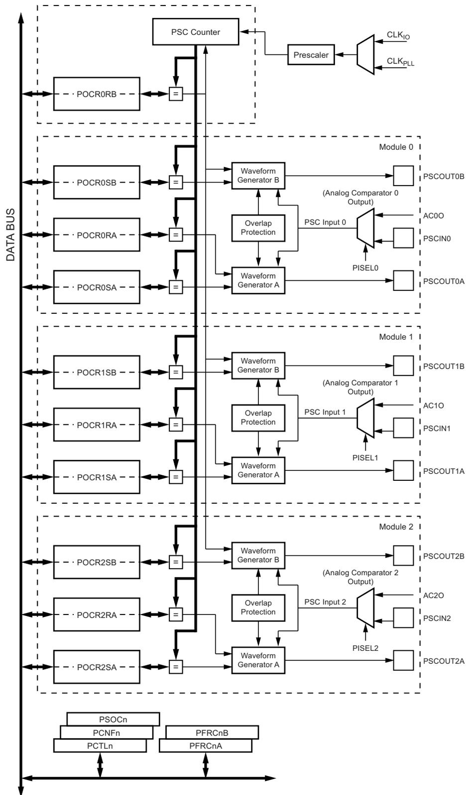
The PSC is based on the use of a free-running 12-bit counter (PSC counter). This counter is able to count up to a top value determined by the contents of POOCR\_RB register and then according to the selected running mode, count down or reset to zero for another cycle.
