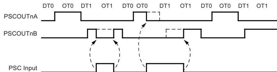
**Figure 14-13. PSC Behavior versus PSCn Input A or Input B in Fault Mode 4**
