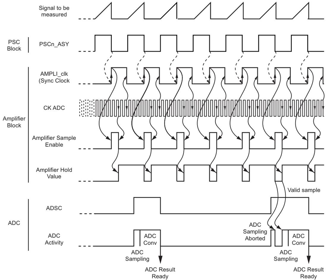
In order to have a better understanding of the functioning of the amplifier synchronization, a timing diagram example is shown [Figure 18-15 on page 215](#).
