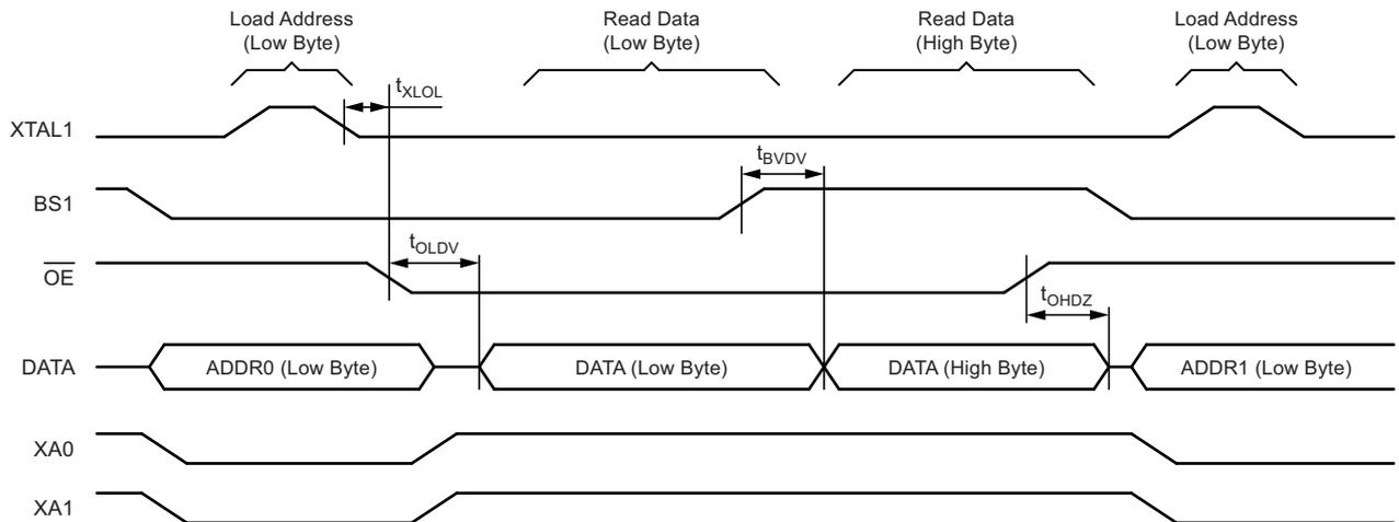
Note: 1. The timing requirements shown in Figure 25-7 (i.e.,  $t_{DVXH}$ ,  $t_{XHXL}$ , and  $t_{XLDX}$ ) also apply to reading operation.
