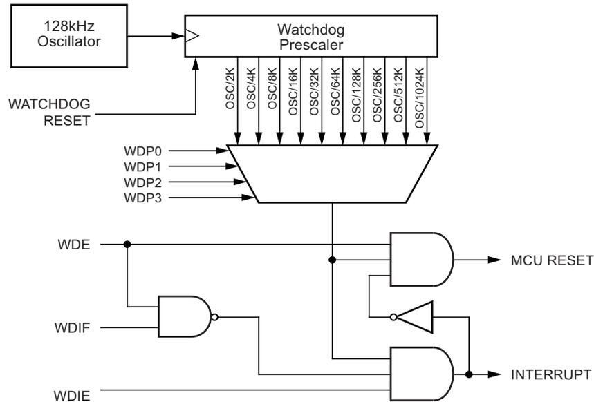
The watchdog timer (WDT) is a timer counting cycles of a separate on-chip 128 kHz oscillator. The WDT gives an interrupt or a system reset when the counter reaches a given time-out value. In normal operation mode, it is required that the system uses the WDR - Watchdog Timer Reset - instruction to restart the counter before the time-out value is reached. If the system doesn't restart the counter, an interrupt or system reset will be issued.
