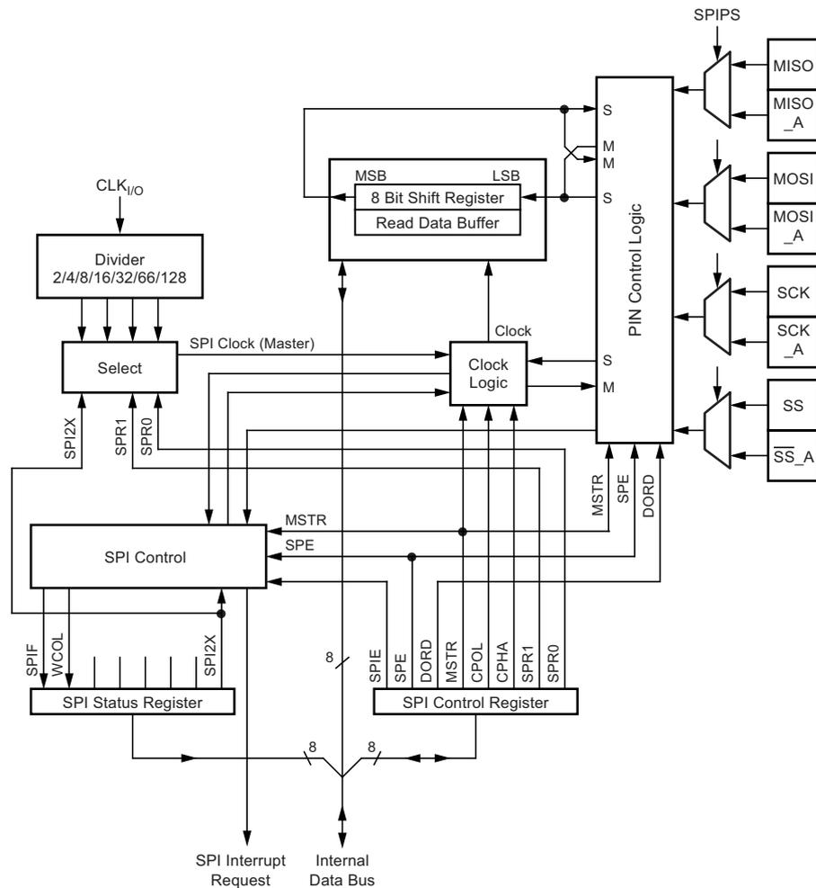
Note: 1. Refer to [Figure 1-1 on page 3](#), and [Table 9-3 on page 58](#) for SPI pin placement.
