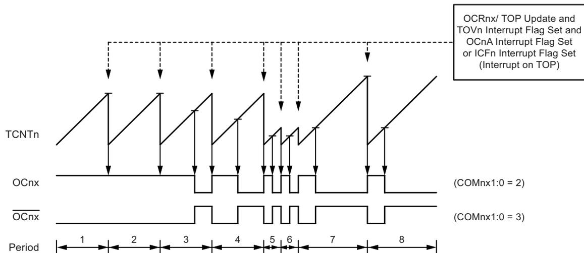
The Timer/Counter overflow flag (TOVn) is set each time the counter reaches TOP. In addition the OCnA or ICFn Flag is set at the same timer clock cycle as TOVn is set when either OCRnA or ICRn is used for defining the TOP value. If one of the interrupts are enabled, the interrupt handler routine can be used for updating the TOP and compare values.
