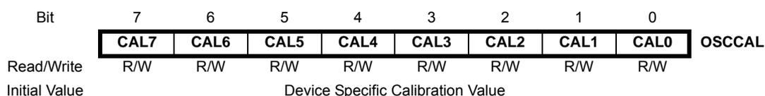
• **Bits 7..0 – CAL7..0: Oscillator Calibration Value**
