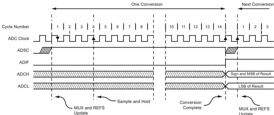
**Figure 18-6. ADC Timing Diagram, Auto Triggered Conversion**
