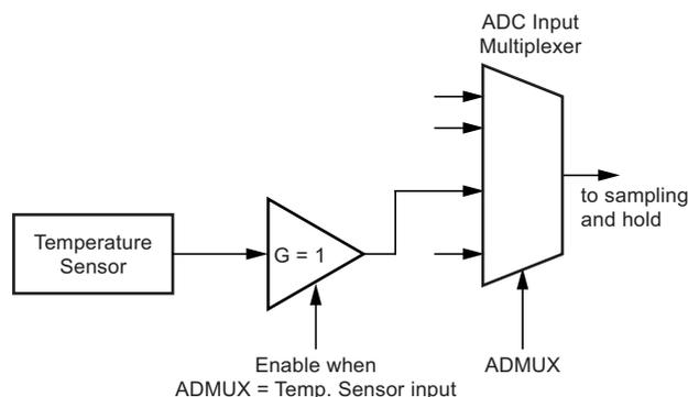
The measured voltage has a linear relationship to the temperature as described in [Table 18-3](#). The voltage sensitivity is approximately 2.5mV/°C and the accuracy of the temperature measurement is ±10°C after bandgap calibration.
