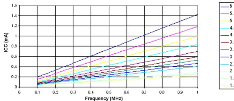
Figure 27-2. Active Supply Current versus Frequency (1 to 24MHz)
