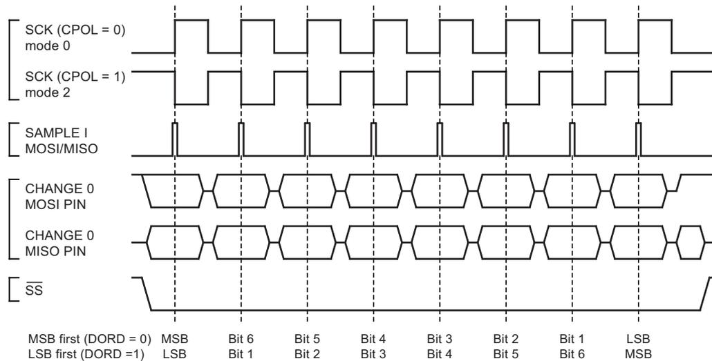
**Figure 15-4. SPI Transfer Format with CPHA = 1**
