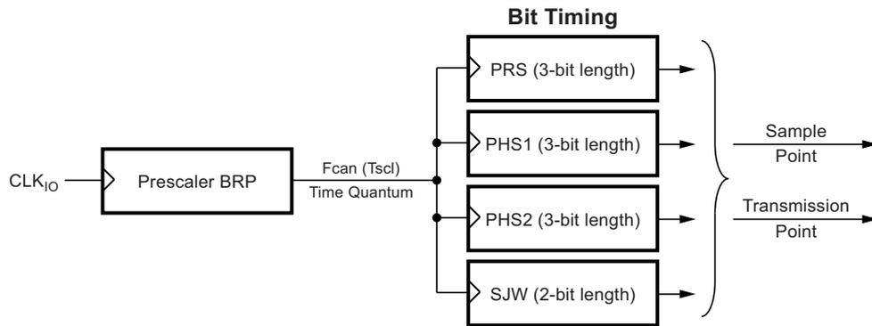
**Figure 16-8. General Structure of a Bit Period**
