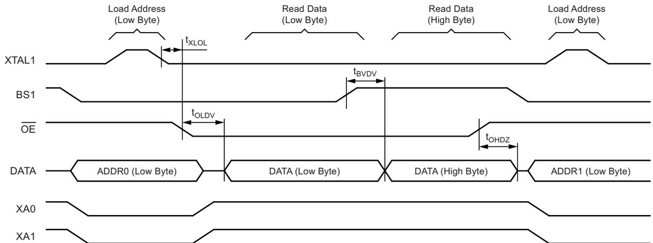
Note: 1. The timing requirements shown in [Figure 25-7 on page 268](#) (i.e.,  $t_{DVXH}$ ,  $t_{XHXL}$ , and  $t_{XLDX}$ ) also apply to reading operation.
