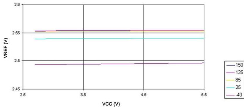
Figure 27-30. VREF Voltage versus Temperature
