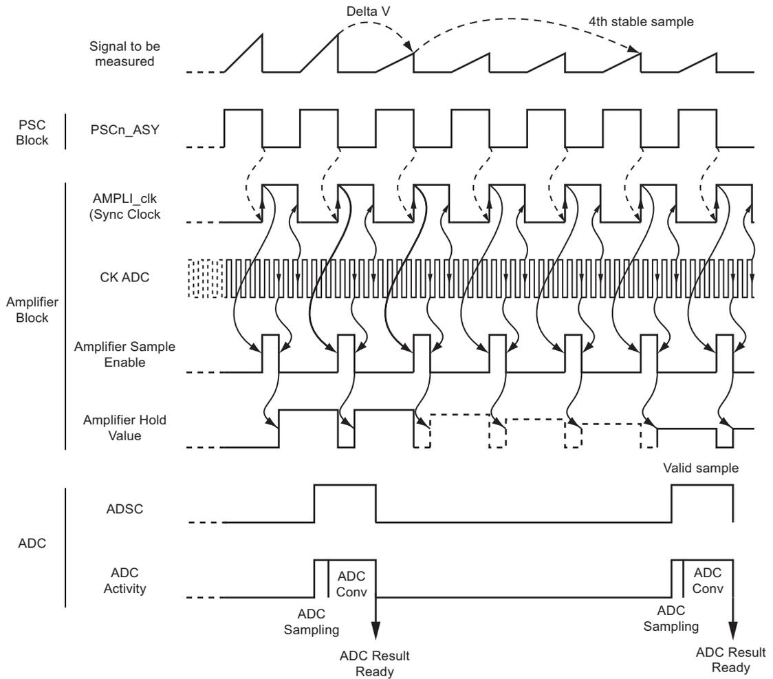
**Figure 18-16. Amplifier Synchronization Timing Diagram**
