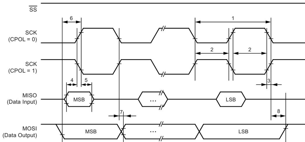
**Figure 26-4. SPI Interface Timing Requirements (Slave Mode)**
