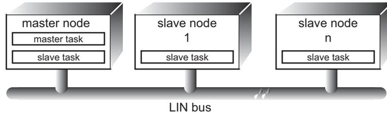
The master task decides when and which frame shall be transferred on the bus. The slave tasks provide the data transported by each frame. Both the master task and the slave task are parts of the Frame handler
