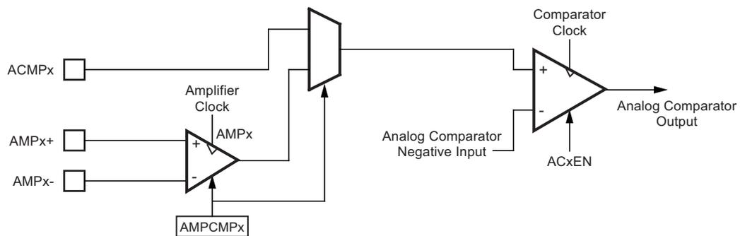
The amplifier clock comes from the ADC and is equal to the ADC Clock divided by 8.
