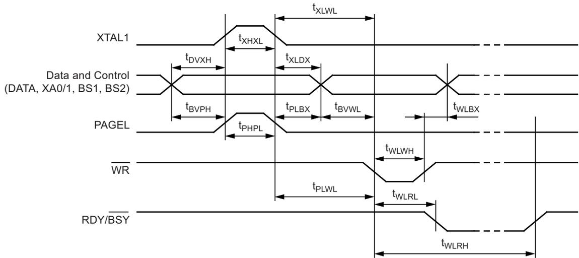
Figure 25-8. Parallel Programming Timing, Loading Sequence with Timing Requirements<sup>(1)</sup>
