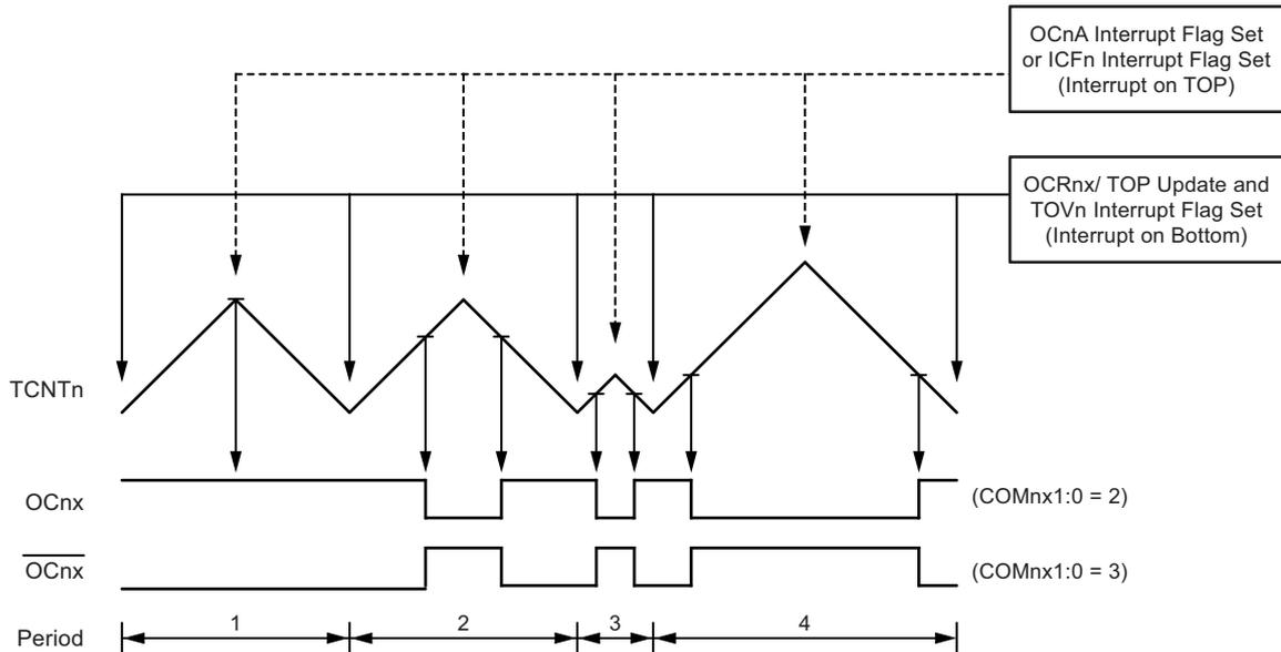
The Timer/Counter overflow flag (TOVn) is set at the same timer clock cycle as the OCRnx registers are updated with the double buffer value (at BOTTOM). When either OCRnA or ICRn is used for defining the TOP value, the OCnA or ICFn flag is set when TCNTn has reached TOP. The interrupt flags can then be used to generate an interrupt each time the counter reaches the TOP or BOTTOM value.
