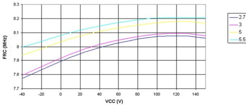
Figure 27-33. Calibrated 8MHz RC Oscillator Frequency versus V<sub>CC</sub>
