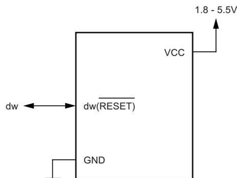
Figure 23-1 shows the schematic of a target MCU, with debugWIRE enabled, and the emulator connector. The system clock is not affected by debugWIRE and will always be the clock source selected by the CKSEL Fuses.
