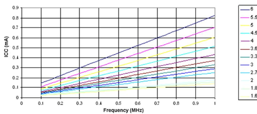
Figure 27-6. Idle Supply Current versus Frequency (1 to 24MHz)
