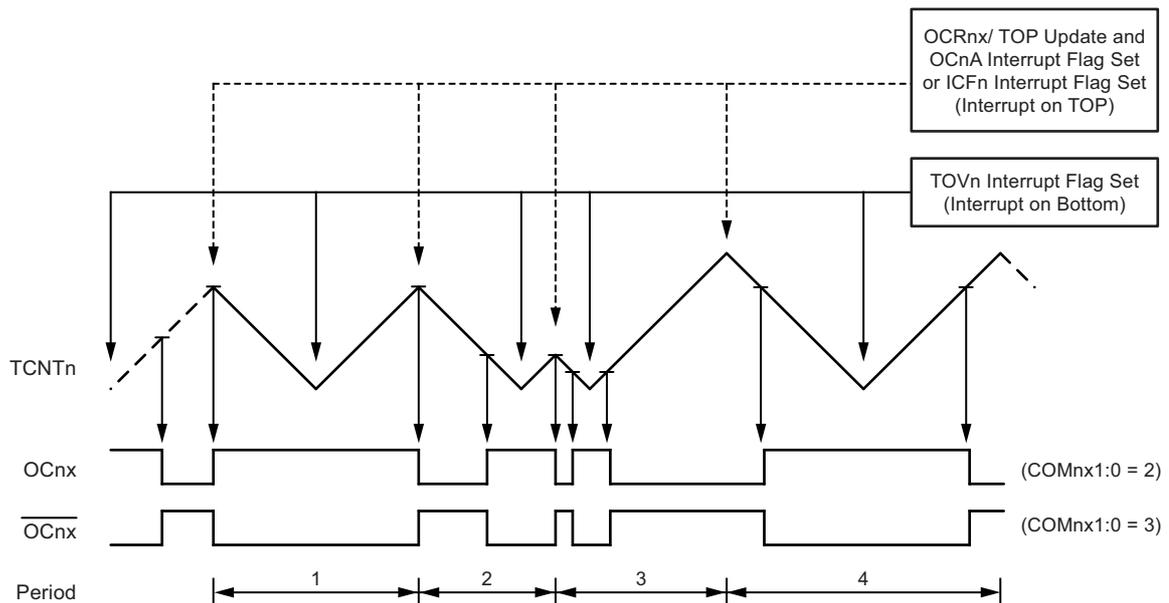
The Timer/Counter overflow flag (TOVn) is set each time the counter reaches BOTTOM. When either OCRnA or ICRn is used for defining the TOP value, the OCnA or ICFn flag is set accordingly at the same timer clock cycle as the OCRn registers are updated with the double buffer value (at TOP). The interrupt flags can be used to generate an interrupt each time the counter reaches the TOP or BOTTOM value.
