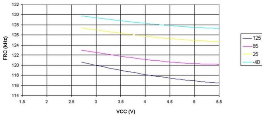
Figure 27-32. Calibrated 8MHz RC Oscillator Frequency versus Temperature
