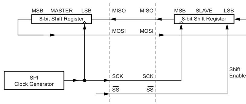
The system is single buffered in the transmit direction and double buffered in the receive direction. This means that bytes to be transmitted cannot be written to the SPI data register before the entire shift cycle is completed. When receiving data, however, a received character must be read from the SPI data register before the next character has been completely shifted in. Otherwise, the first byte is lost.
