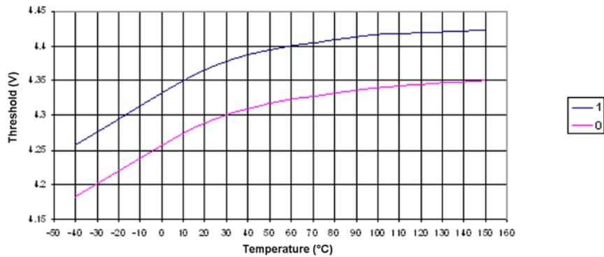
Figure 27-27. BOD Thresholds versus Temperature (BODLEVEL Is 2.7V)
