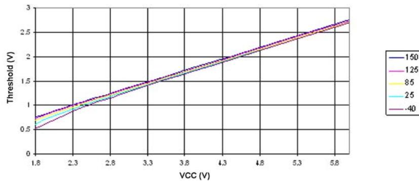
Figure 27-21. I/O Pin Input Hysteresis Voltage versus  $V_{CC}$
