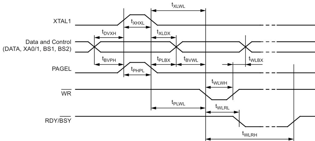
Figure 26-6. Parallel Programming Timing, Loading Sequence with Timing Requirements<sup>(1)</sup>
