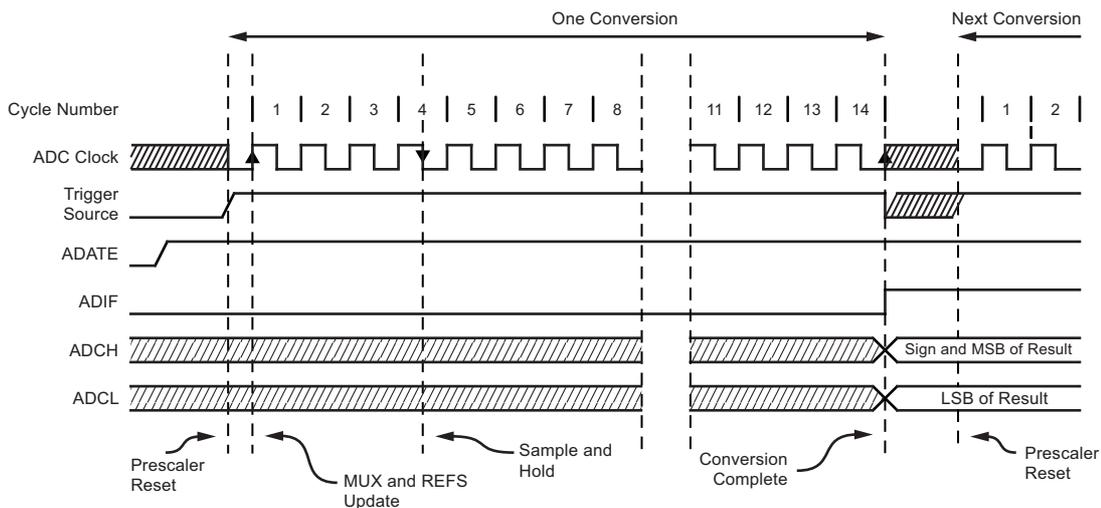
**Figure 18-7. ADC Timing Diagram, Free Running Conversion**
