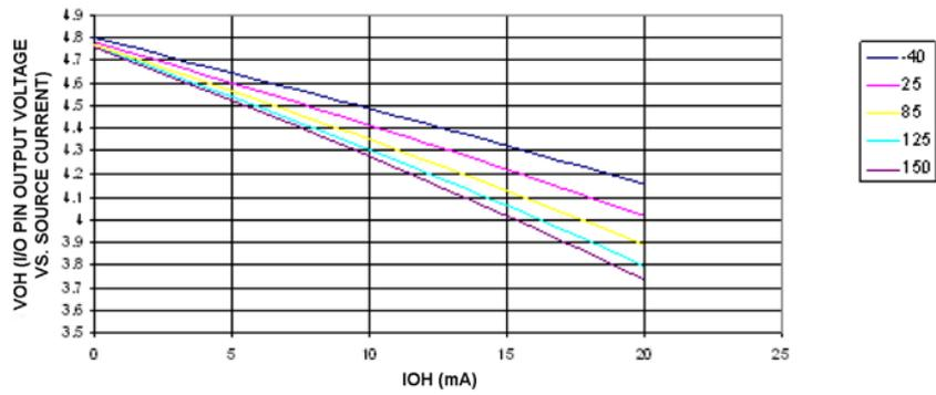
Figure 27-16. I/O Pin Output Voltage versus Source Current ( $V_{CC} = 3V$ )
