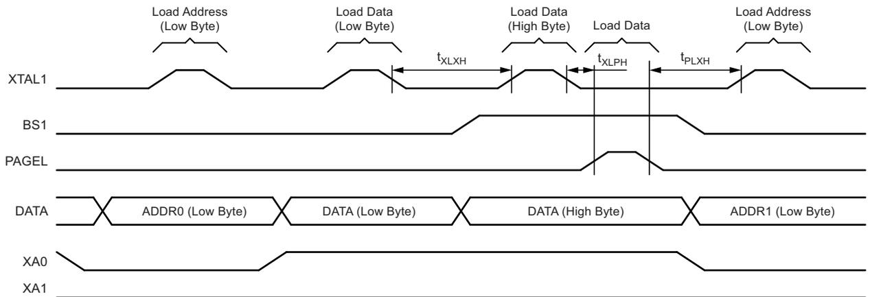
Note: 1. The timing requirements shown in Figure 25-7 (i.e.,  $t_{DVXH}$ ,  $t_{XHXL}$ , and  $t_{XLDX}$ ) also apply to loading operation.
