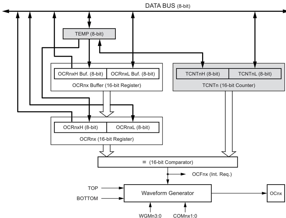
The OCRnx register is double buffered when using any of the twelve *Pulse Width Modulation* (PWM) modes. For the normal and *Clear Timer on Compare* (CTC) modes of operation, the double buffering is disabled. The double buffering synchronizes the update of the OCRnx compare register to either TOP or BOTTOM of the counting sequence. The synchronization prevents the occurrence of odd-length, non-symmetrical PWM pulses, thereby making the output glitch-free.
