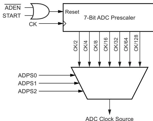
By default, the successive approximation circuitry requires an input clock frequency between 50kHz and 2MHz to get maximum resolution. If a lower resolution than 10 bits is needed, the input clock frequency to the ADC can be higher than 2MHz to get a higher sample rate.
