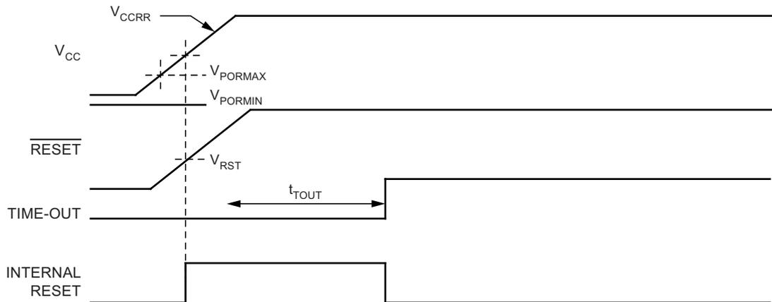
**Figure 7-3. MCU Start-up, RESET Extended Externally**
