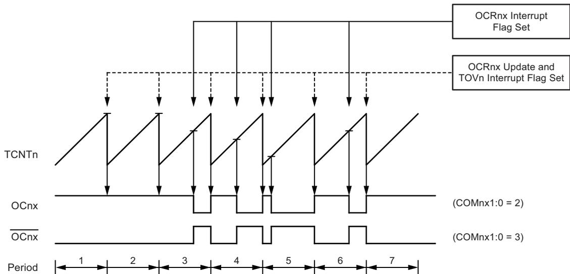
The Timer/Counter overflow flag (TOV0) is set each time the counter reaches TOP. If the interrupt is enabled, the interrupt handler routine can be used for updating the compare value.
