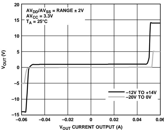
Figure 21. Source and Sink Capability of Output Amplifier
