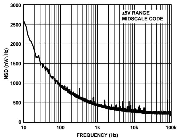
Figure 24. Noise Spectral Density (NSD) vs. Frequency
