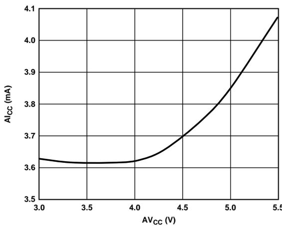
Figure 27. Supply Current in Normal Mode ( $A_{LCC}$ ) vs. Supply Voltage ( $A_{VCC}$ )
