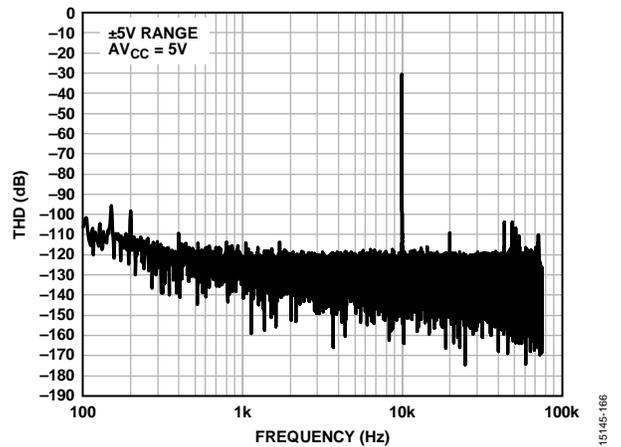
Figure 40. Total Harmonic Distortion (THD) vs. Frequency
