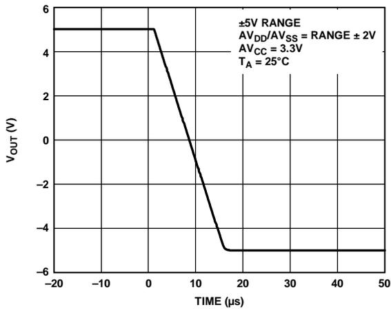
Figure 20. Full-Scale Settling Time (Falling Voltage Step)
