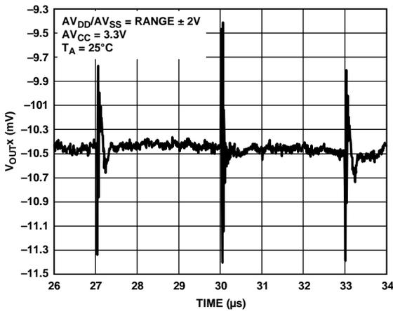
Figure 26. Digital Feedthrough for LFCSP Package
