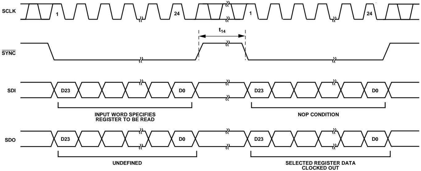
Figure 4. Readback Timing Diagram
