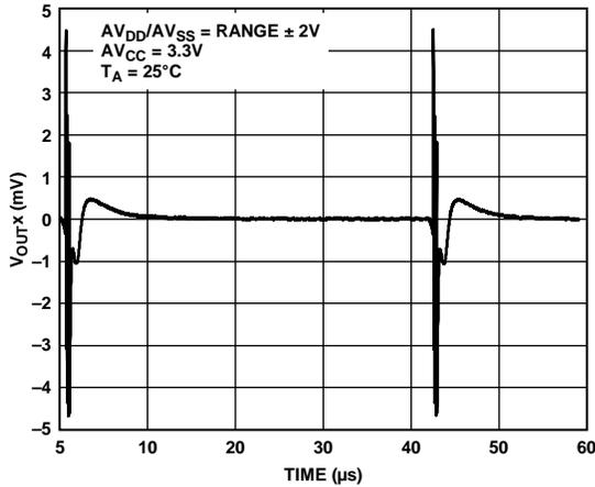
Figure 25. Digital Feedthrough for WLCSP Package
