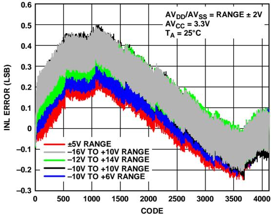
Figure 8. INL Error vs. DAC Code (Bipolar Outputs)
