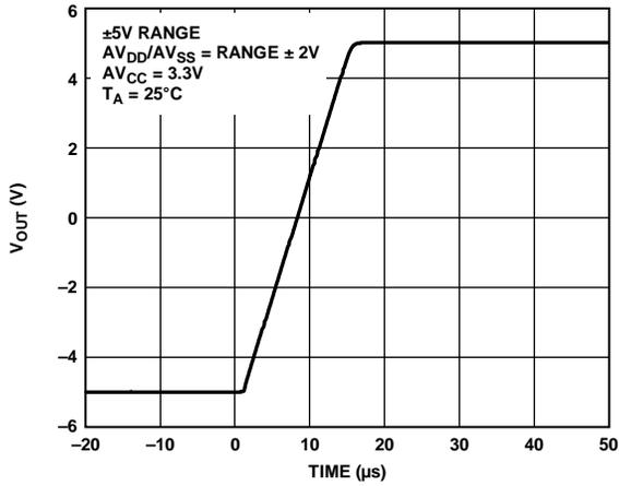
Figure 19. Full-Scale Settling Time (Rising Voltage Step)
