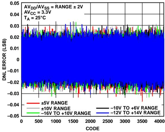
Figure 9. DNL Error vs. DAC Code (Bipolar Outputs)
