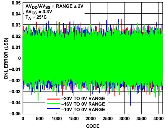
Figure 10. DNL Error vs. DAC Code (Unipolar Outputs)
