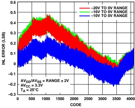
Figure 7. INL Error vs. DAC Code (Unipolar Output)
