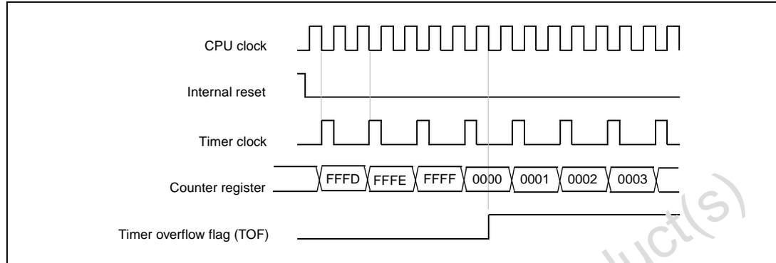
**Figure 43. Counter timing diagram, internal clock divided by 4**
