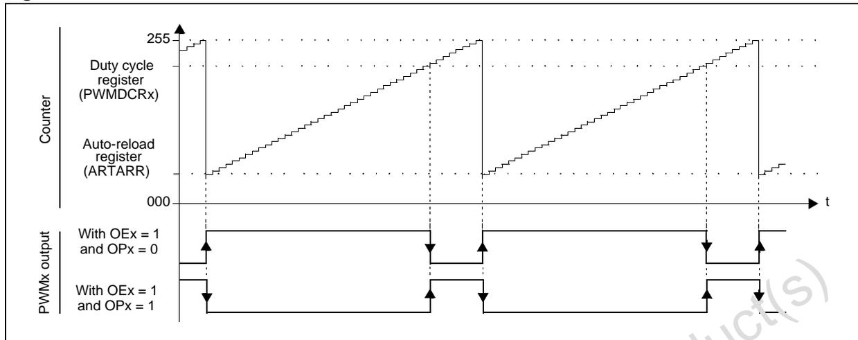
Figure 37. PWM signal from 0% to 100% duty cycle
