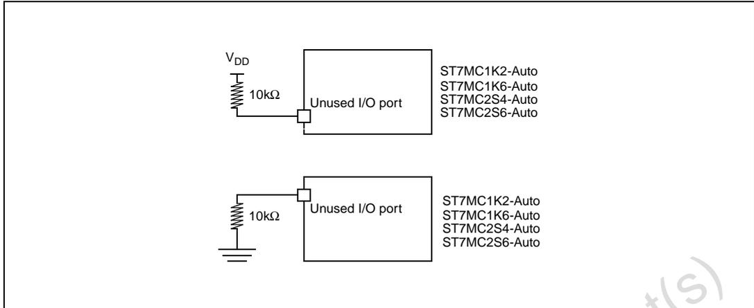
1. I/O can be left unconnected if it is configured as output (0 or 1) by the software. This has the advantage of greater EMC robustness and lower cost.
