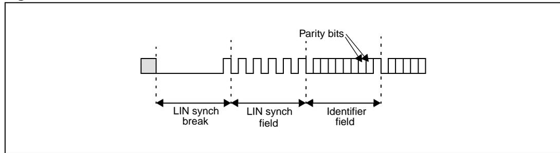
The bits involved are the two MSB positions (7th and 8th bits if M = 0; 8th and 9th bits if M = 0) of the identifier character. The check is performed as specified in Figure 67 by the LIN specification.
