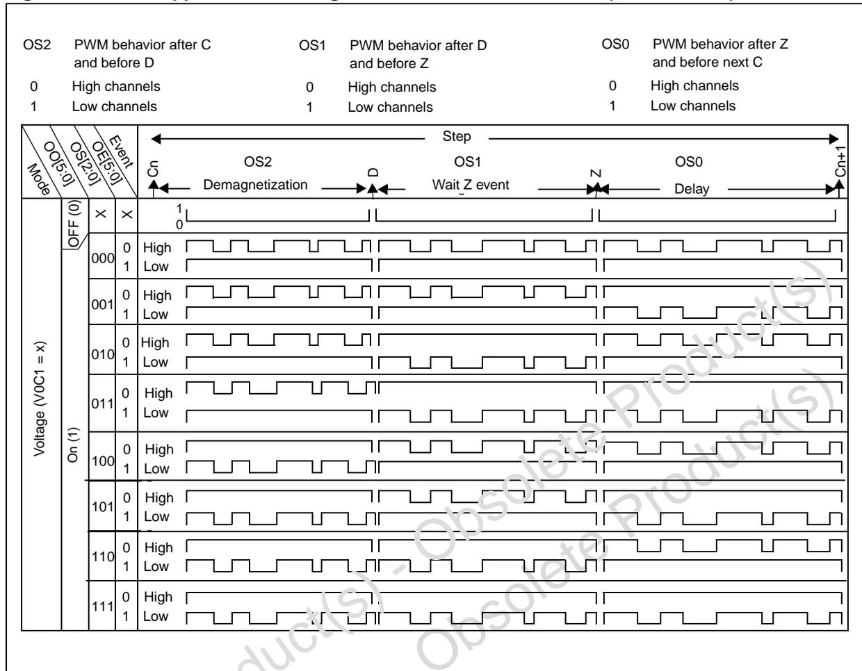
Figure 111. PWM application in voltage or current sensor mode (see Table 134)
