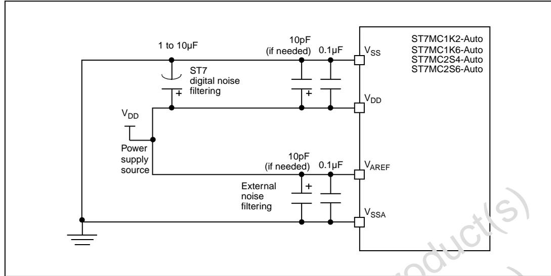
ADC accuracy with  $V_{DD} = 5.0V$
