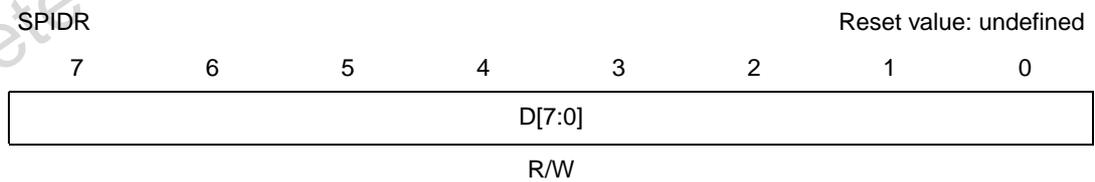
The SPIDR register is used to transmit and receive data on the serial bus. In a master device, a write to this register initiates the transmission/reception of another byte.
