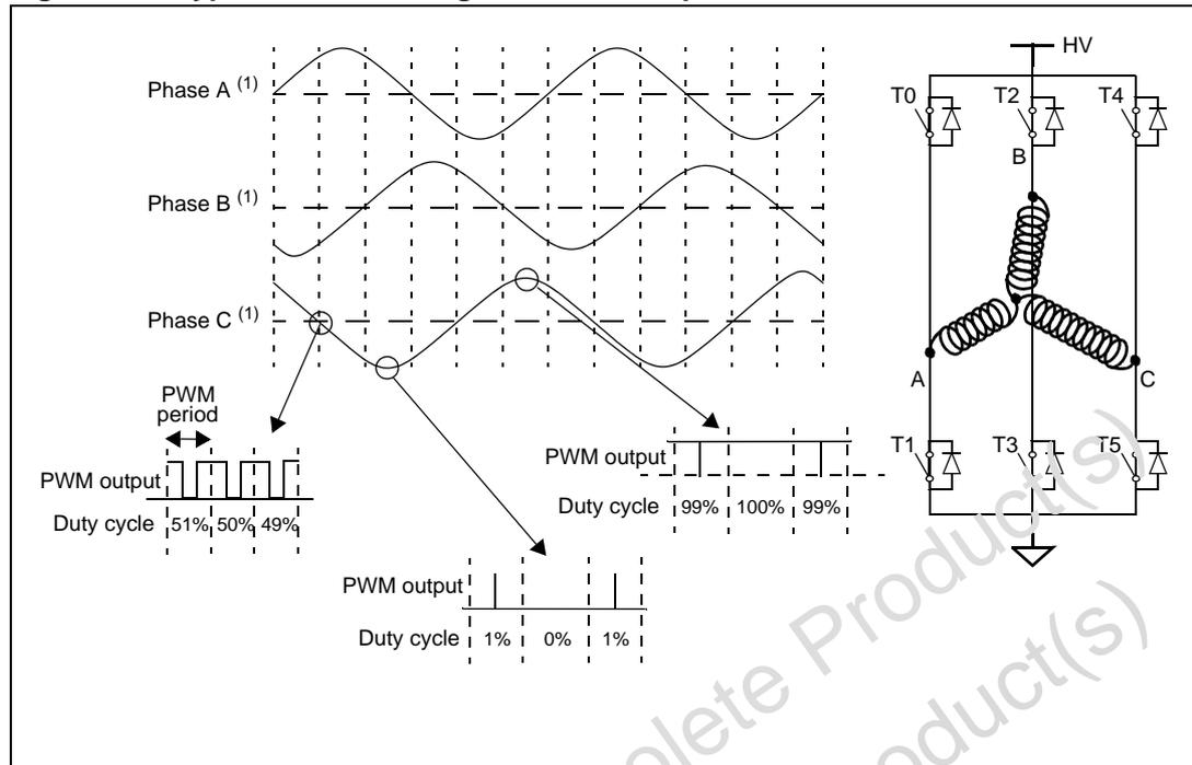
1. These simplified chronograms represent the phase voltages after low-pass filtering of the PWM outputs reference signals.
