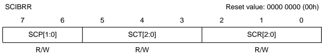
*Note:* When LIN slave mode is disabled, the SCIBRR register controls the conventional baud rate generator.
