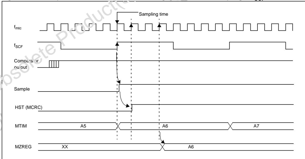
**Figure 153. Example 3: Waveforms for zero-crossing detection with sampling after a delay during PWM on-time**
