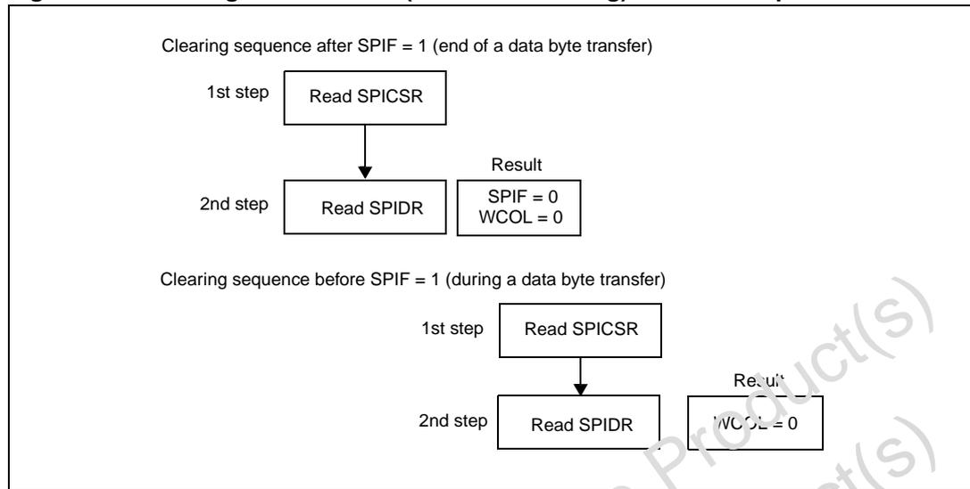
1. Writing to the SPIDR register instead of reading it does not reset the WCOL bit.
