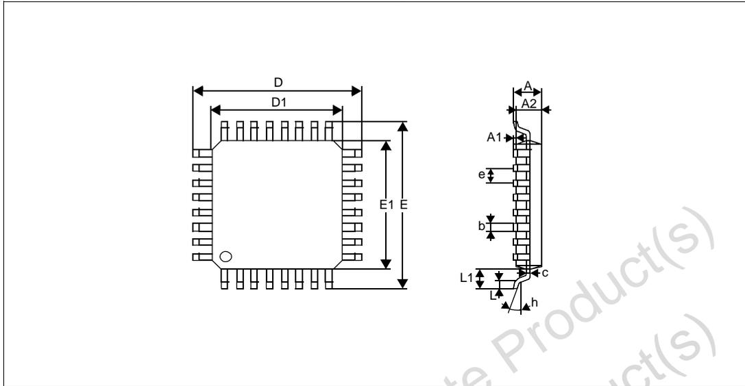
Table 223. 32-pin low profile quad flat package mechanical data
