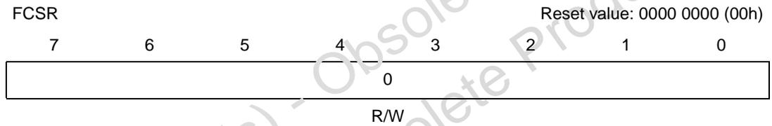
This register is reserved for use by programming tool software. It controls the Flash programming and erasing operations.
