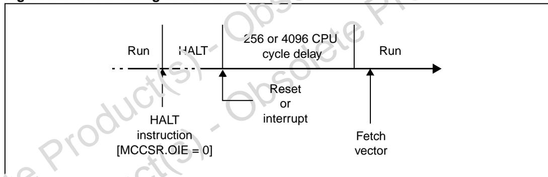
Figure 27. Halt mode flowchart
