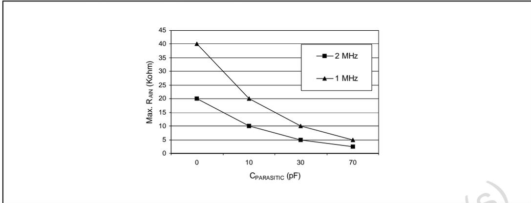
1.  $C_{PARASITIC}$  represents the capacitance of the PCB (dependent on soldering and PCB layout quality) plus the pad capacitance (3pF). A high  $C_{PARASITIC}$  value downgrades conversion accuracy. To remedy this,  $f_{ADC}$  should be reduced.
