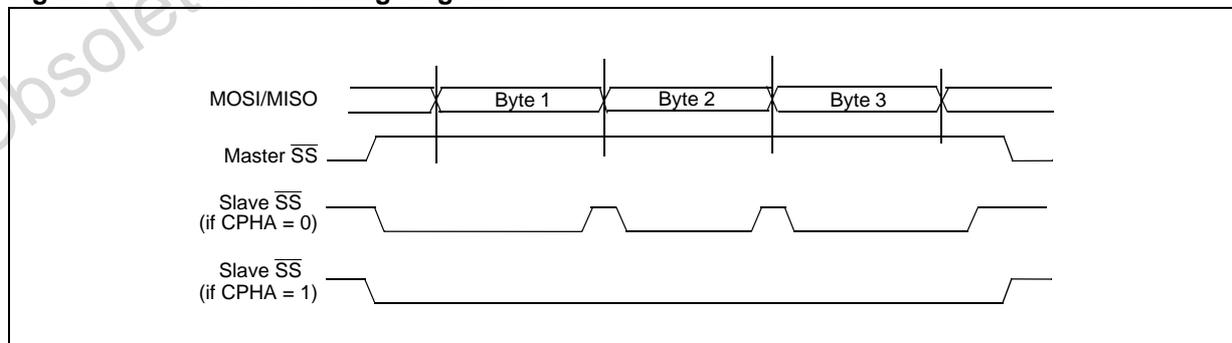
**Figure 57. Hardware/software slave select management**
