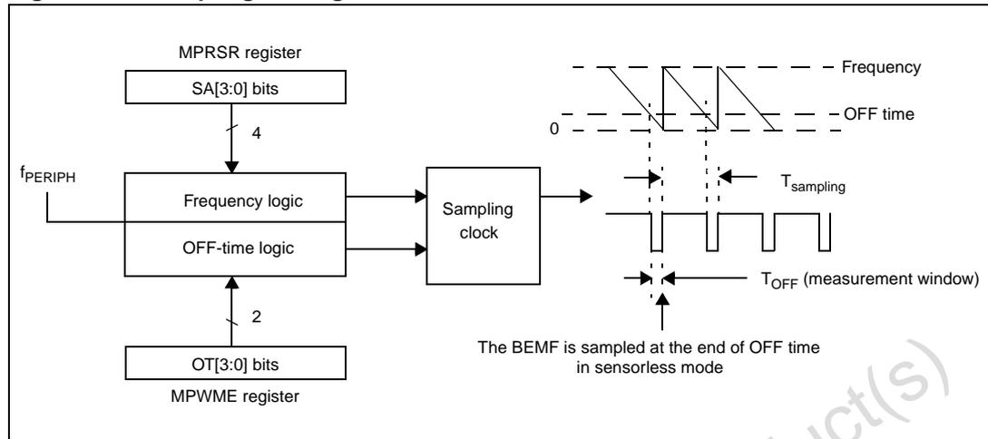
1. The MTC controller input frequency ( $f_{PERIPH}$ ) is 4 MHz in this example, It can be configured to 8 MHz with the XT16: XT8 bits in the MCONF register
