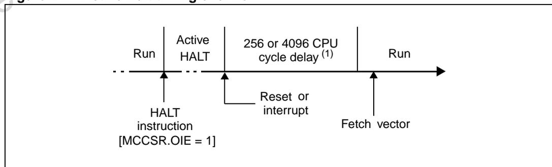
1. This delay occurs only if the MCU exits Active Halt mode by means of a reset.
